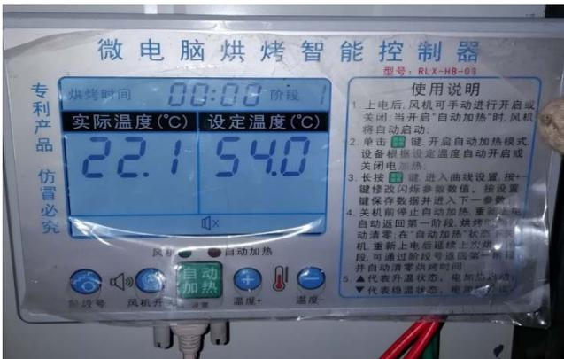
Fig. 26 Temperature and heating controller
